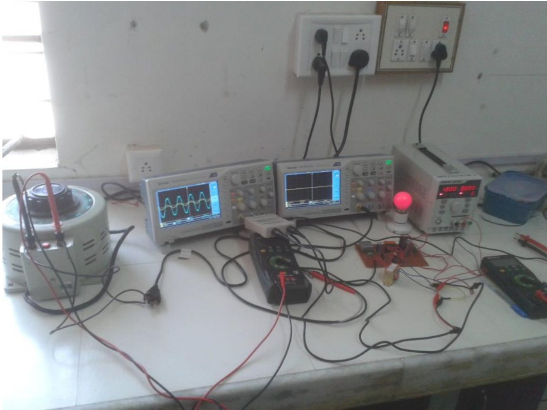
Fig.6.11: With PFC on Breadboard with Bulb Load
