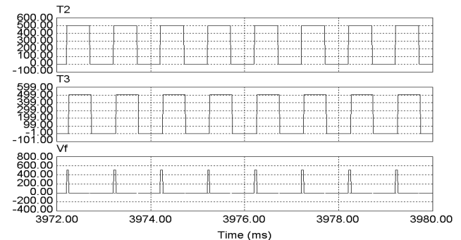
Fig.14 Voltage across the field at 600rpm reference
