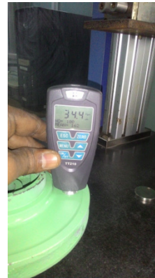
Fig. 3. Coating thickness measurement.
