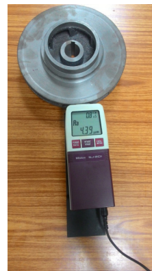
Fig. 4. Surface roughness measurement.
