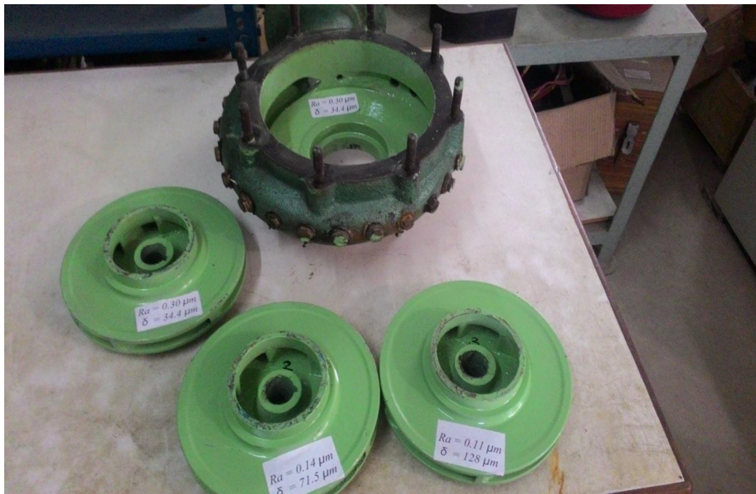
Figure 8.5 Polyurethane coated impeller and volute casing with different coating thickness and surface finish
