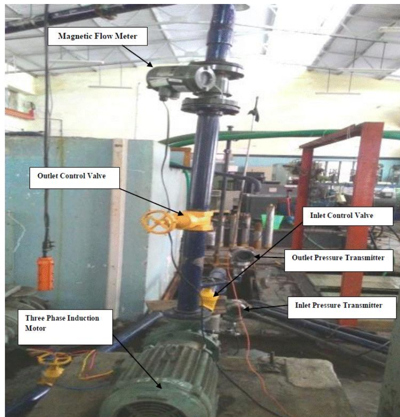
Figure 3.5 (a) Laboratory test setup as per ISO 9906 and IS 11346
