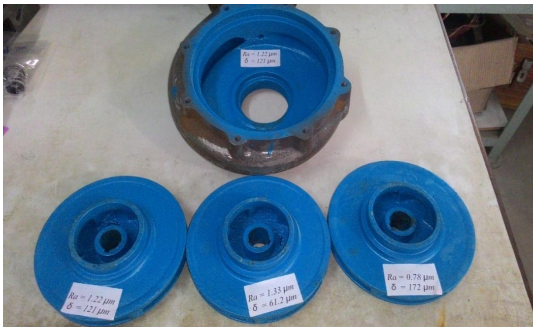
Figure 8.3 Epoxy coated impeller and volute casing with different coating thickness and surface finish
