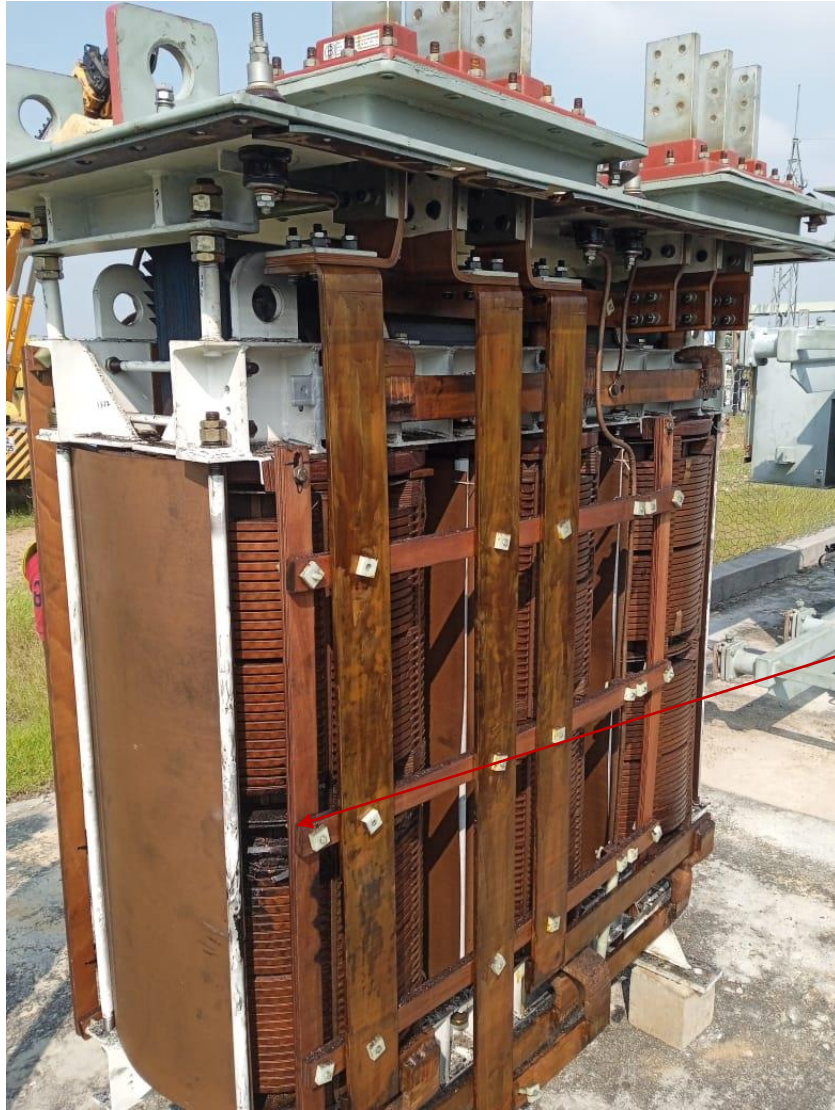
Figure 4(c) 12.5 MVA Inverter Duty Transformer Failure
