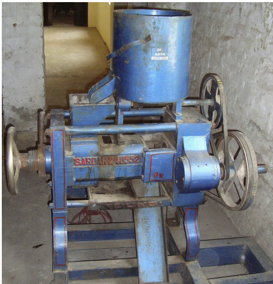
Fig. 1 – Screw press oil expeller.
