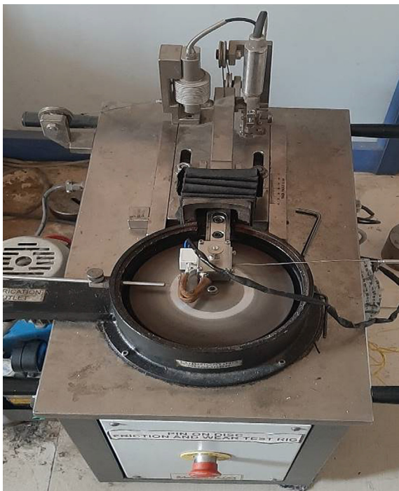
Fig. 1. Schematic diagram of Pin-on-Disc Tribometer.
