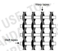
IS 16187:2014 prescribes the manufacturing and technical requirements for high density polyethylene (HDPE)/polypropylene (PP) leno woven sacks for packaging and storage of fruits and vegetables. This standard covers requirements for Type 1 and Type 2 sacks having nominal holding capacities of 25 kg and 50 kg, respectively. It also prescribes method of sampling, criteria for conformity, tests and requirements for labelling and marking.
