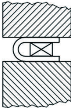
Figure — Bending the Legs of the Test Piece
