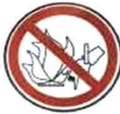
WATER AS EXTINGUISHING AGENT PROHIBITED
