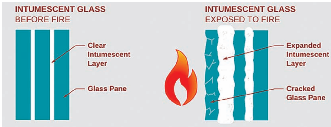
FIG. 60 INTUMESCENT-LAYER TYPE FIRE-RESISTANT GLASS
