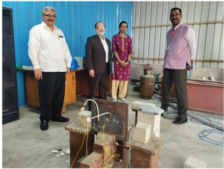
(The rudimentary LPG-based set-up is proposed to be engineered further and scaled to connect with the regular structural engineering testing machines to carry out a combination of regular loads and fire on real-scale elements to evaluate their performance.)
