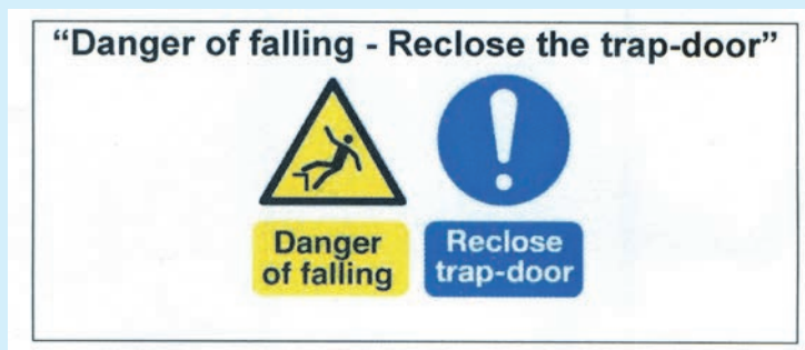
FIG. 5 TYPICAL NOTICE ON TRAP DOORS
