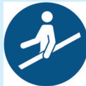
FIG. 16 MANDATORY ACTION SIGN 'USE THE HANDRAIL'
