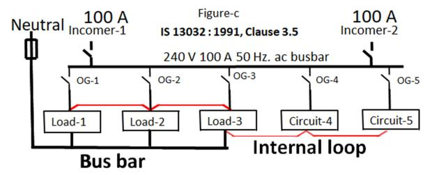
1. More than one or all outgoing circuits could be looped with a single neutral at load circuit irrespective of the current rating of the loads from an SPN OR TPN MCBDB (refer to Figure-c). This may overheat that neutral wire towards an undesired event of electrical fire hazard.
