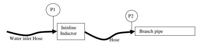
1) Branch pipe with inlet pressure of 7 kg/sqcm.
