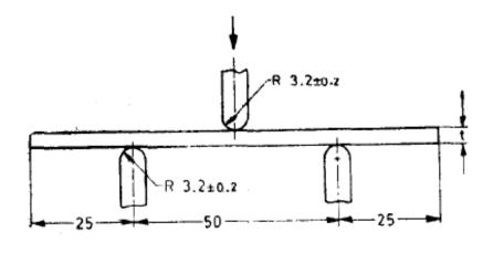
t = Thickness of SpecimenAll dimensions in millimetres.
