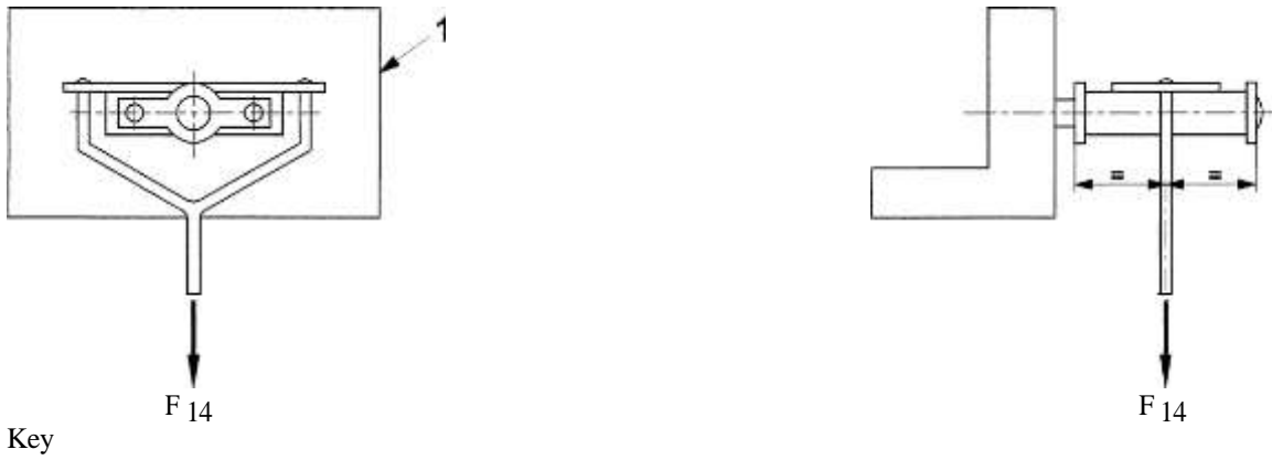
FIG. 38 PEDAL/PEDAL-SPINDLE ASSEMBLY: STATIC STRENGTH TEST
