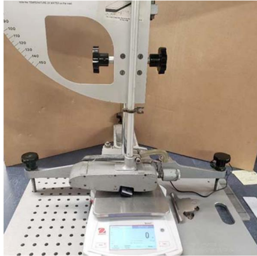
FIG. 6 ARRANGEMENT OF THE BRITISH PENDULUM TESTER, SHOWING PENDULUM ASSEMBLY AND ELECTRONIC SCALE WITH BEARING PLATE USED TO MEASURE SLIDER LOAD
