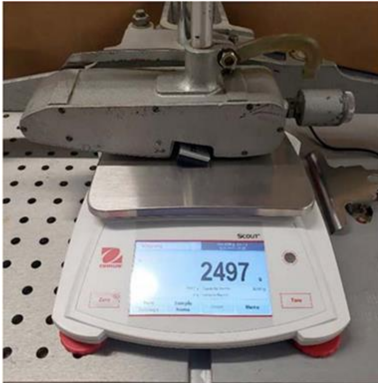
FIG. 8 POSITION OF THE PENDULUM AND RUBBER SLIDER AFTER SPACER IS REMOVED DURING CALIBRATION PROCEDURE
