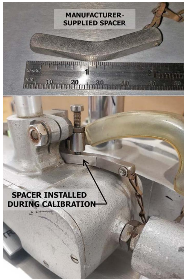
FIG. 7 MANUFACTURER-SUPPLIED SPACER AND LOCATION OF SPACER WHEN INSERTED DURING THE CALIBRATION PROCEDURE
