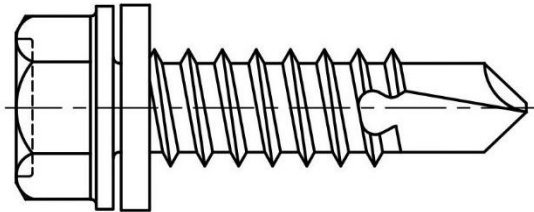
FIG. 1(A) WASHER HEAD WITH CAPTIVE WASHER
