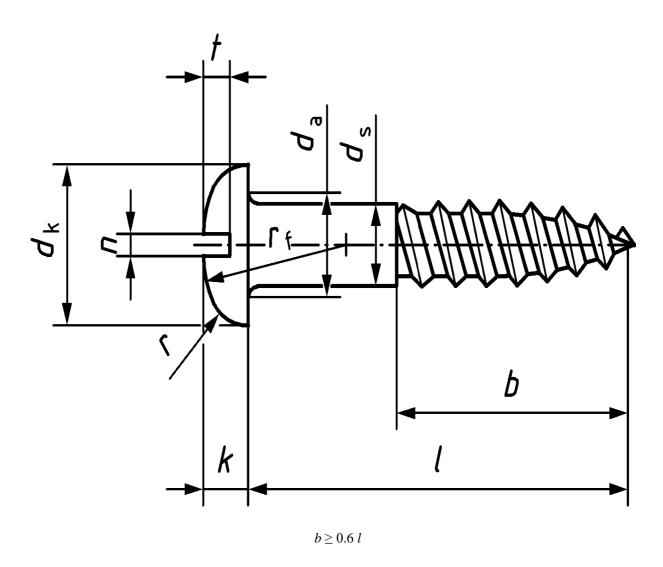
FIG. 1 DIMENSIONS OF SLOTTED ROUND HEAD WOOD SCREWS
