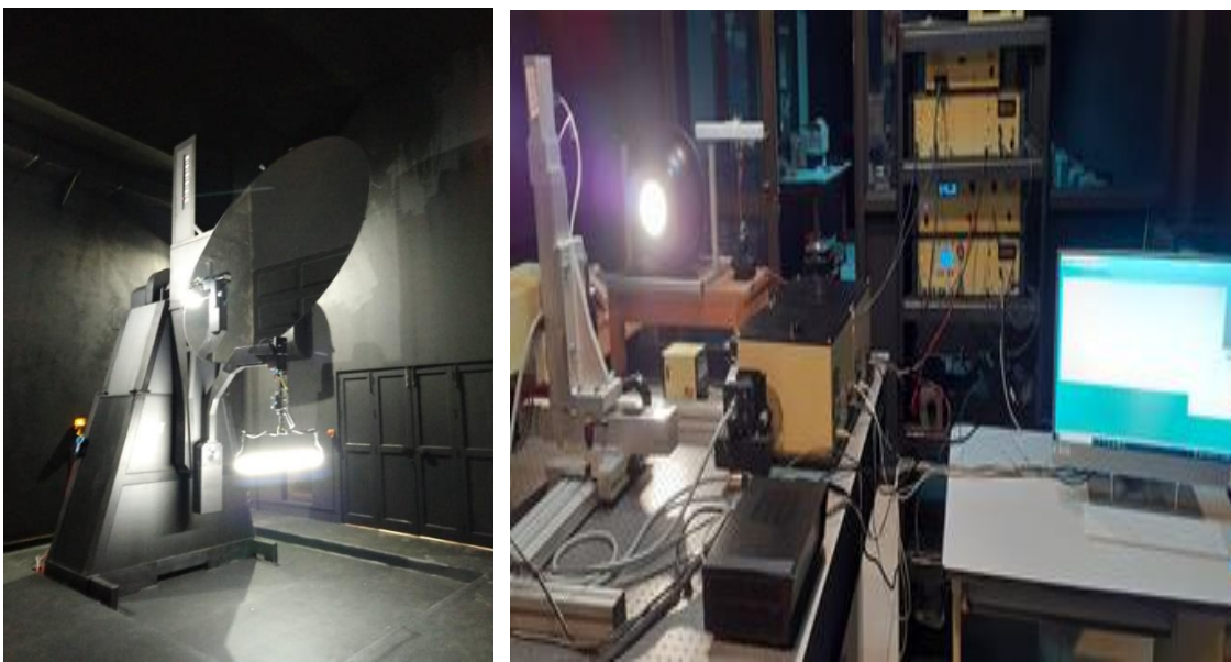
FIG. 13 C-TYPE GONIOPHOTOMETER SYSTEM AND PHOTO BIOLOGICAL SAFETY TESTING SYSTEM ESTABLISHED RECENTLY AT CSIR-NPL
