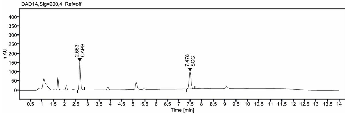
Representative Chromatogram of a 0.20 mg/mL coco amido propyl betaine and sodium cocoyl glycinate mixed reference standard on YMC pack ODS column.
