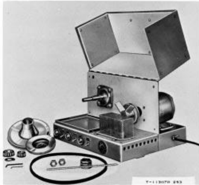
FIG. 1 APPARATUS FOR TESTING LEAKAGE TENDENCIES OF WHEEL BEARING GREASES
