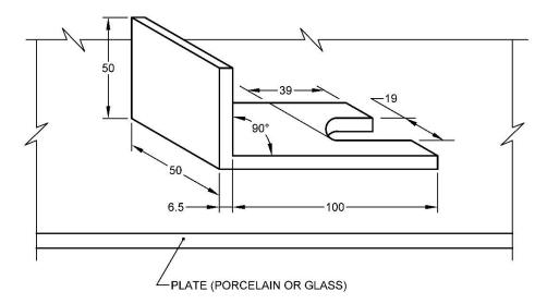
NOTE - TOLERANCE ON ALL DIMENSIONS SHALL BE ±0.2 mm.
