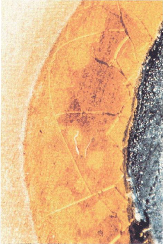
a) Brownish-green flux residue but no evidence of corrosion growth: No Corrosion
