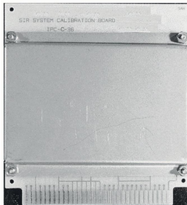
FIG. 12 RESISTOR VERIFICATION BOARD WITH PROTECTIVE COVER
