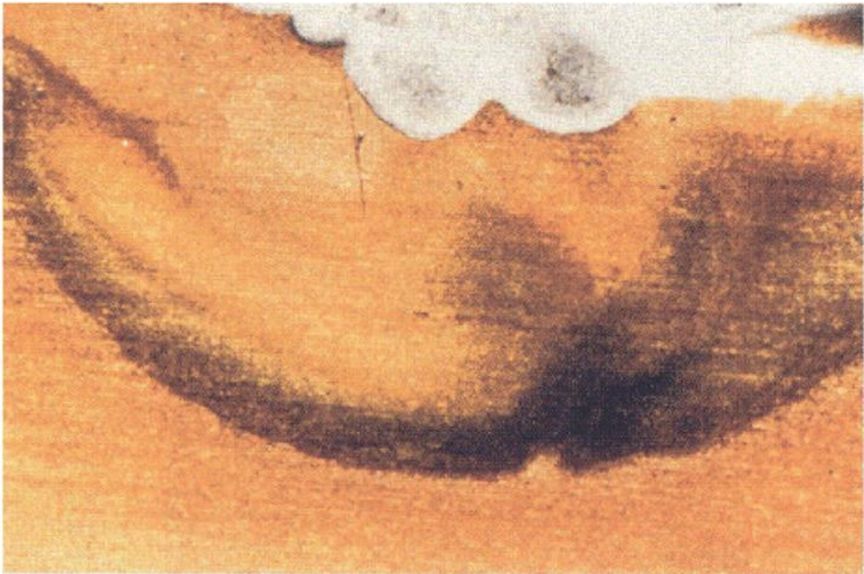
b) Olive-green flux residue due to copper salts, but no evidence of corrosion growth: No Corrosion
