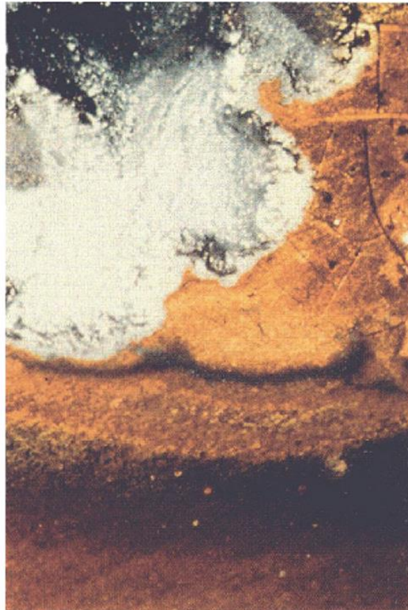
c) Corrosion product growth (blue spots) at the flux/copper boundary: Minor Corrosion
