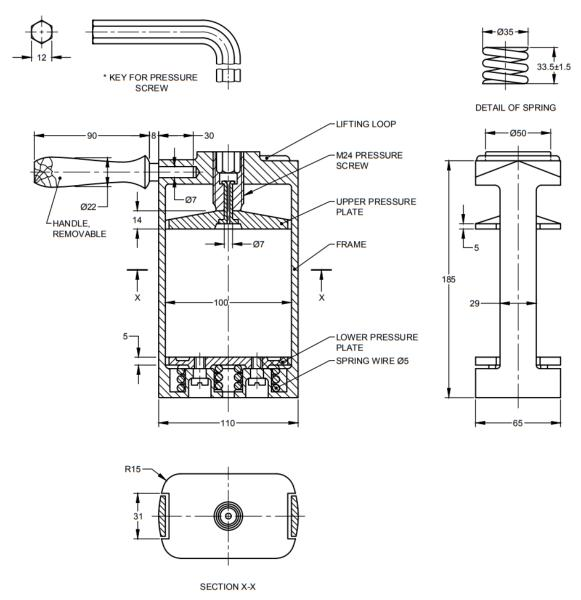
\*See IS 3082 All dimensions in millimetres. Fig. 1 Clamp, Flask, Dental
