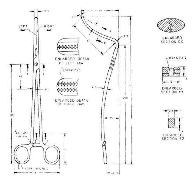
All dimensions in millimetres. FIG. 1 AORTIC CLAMP
