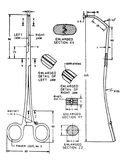
All dimensions in millimetres. FIG. 1 CLAMP, ATRIAL PRRENDAGE, GLOVER'S PATTERN
