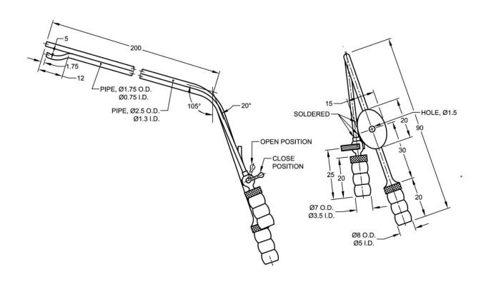
All dimensions in millimeters. FIG. 1 SUCTION IRRIGATION CANNULA WITH LOCKING DEVICE
