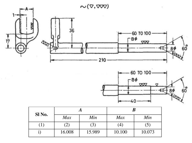
NOTE — Tolerance for untoleranced dimensions shall conform to fine grade deviation of IS 2102 (Part 1)/ ISO 2768-1 and IS 17894/ISO 22081.
