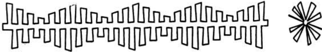
FIG. 3 TYPICAL TWISTED FORM OF TANG BAR
