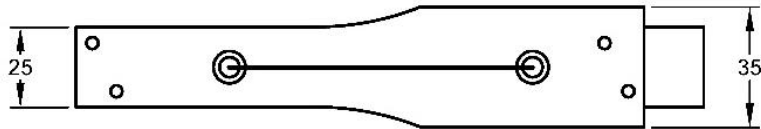
All dimensions in millimeters. FIG.4 (C) FRAME SIDE BAR
