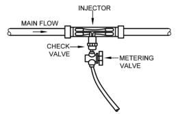
INSTALLED IN THE MAIN FLOW LINE TOTAL FLOW OF THE SYSTEM GOES THROUGH THE INJECTOR.
