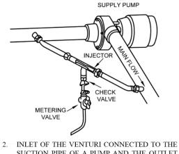
2. INLET OF THE VENTURI CONNECTED TO THE SUCTION PIPE OF A PUMP AND THE OUTLET CONNECTED TO THE DELIVERY PIPE OF THE PUMP. PRESSURE DIFFERENTIAL IS CREATED AUTOMATICALLY WHEN THE PUMP STARTS RUNNING.
