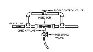
3. INJECTOR CAN BE INSTALLED DIECTLY IN THE MAIN LINE WITH A BY-PASS CONNECTION HAVING FLOW CONTROL VALVE. WHEN INJECTION IS NOT REQUIRED MAIN FLOW CAN BE DIVERTED THROUGH THE BY-PASS IN TO THE SYSTEM.
