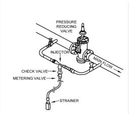
1. A REGULAR VALVE INSTALLED IN BETWEEN THE INLET AND OUTLET CONNECTIONS OF THE VENTURI INJECTOR CREATES DIFFERENTIAL PRESSURE AND FINALLY VACUUM NEAR THE SUCTION PORT.
