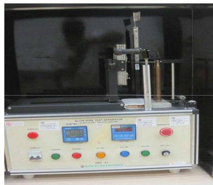
Fig. 19 Glow Wire Test Set Up
