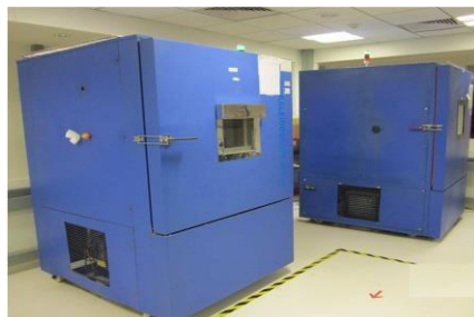
Fig. 21 Typical Humidity Chamber
