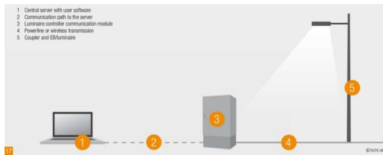
Fig. 3 Examples of Components of a Powerline or Wireless Lighting Management System
