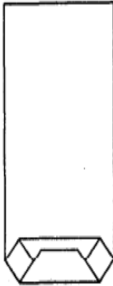
Fig. 4 Open Mouth-Pasted-Flat-Hexagonal Bottom Sack
