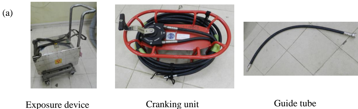
FIG. 1 (a) PHOTOGRAPH OF A CO-60 GAMMA CAMERA WITH CRANKING UNIT AND GUIDE TUBE
