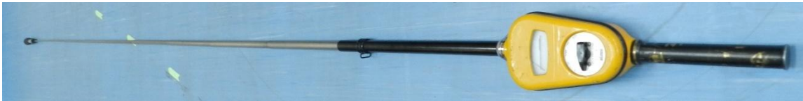
FIG. 2 COMMONLY USED DETECTOR (TELETECTOR) IN INDUSTRIAL RADIOMETRY
