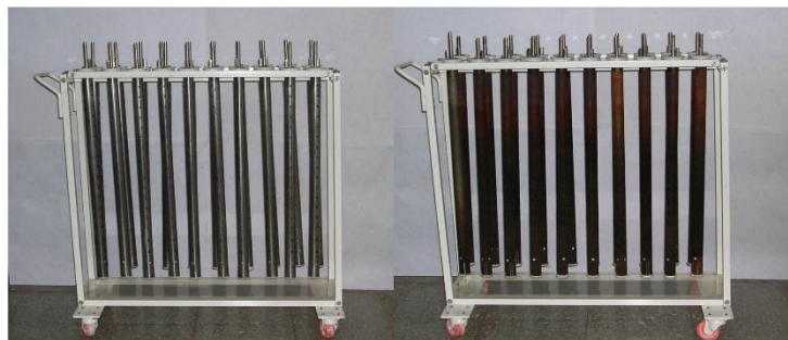
FIG. 3 CATHODE WITH AND WITHOUT DEVELOPMENT
