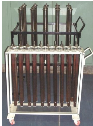
FIG. 2 ANODE AND DEVELOPED CATHODE ELECTROLYTIC CELL
