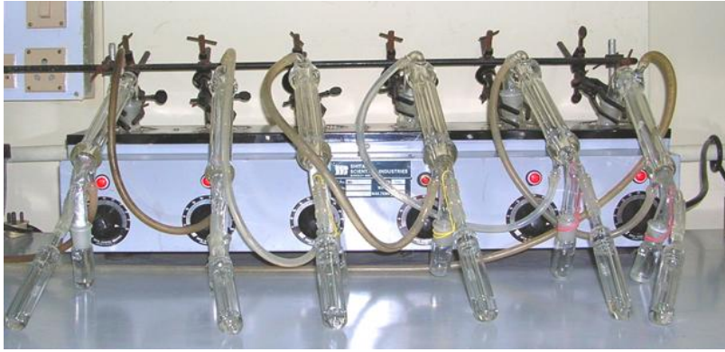
FIG. 5 NEUTRALISATION SETUP FOR SAMPLES POST ELECTROLYSIS
