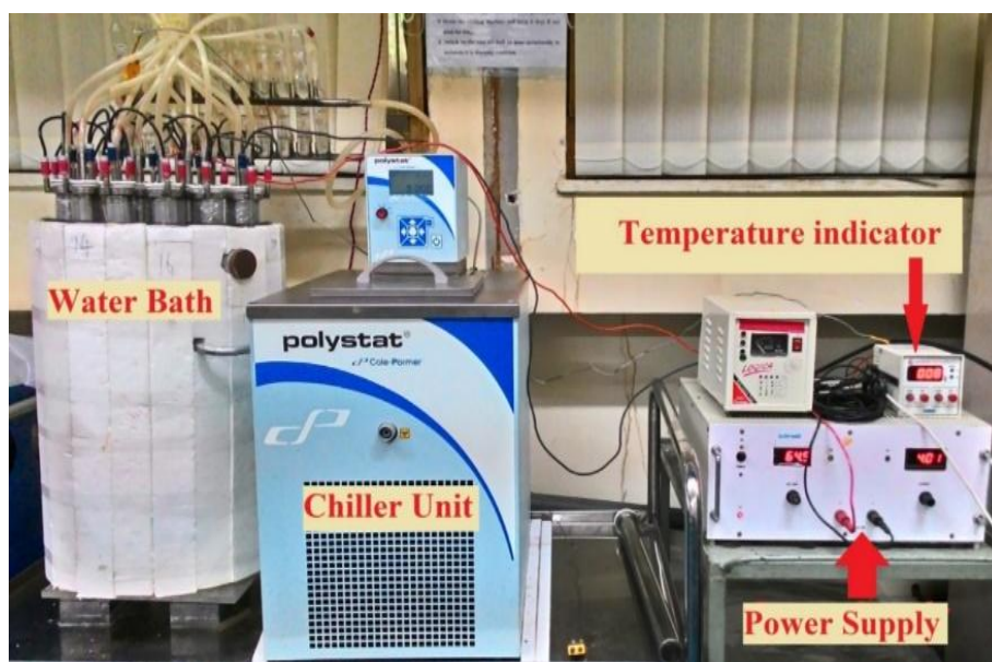
Fig. 4 ELECTROLYSIS SETUP FOR TRITIUM ENRICHMENT
