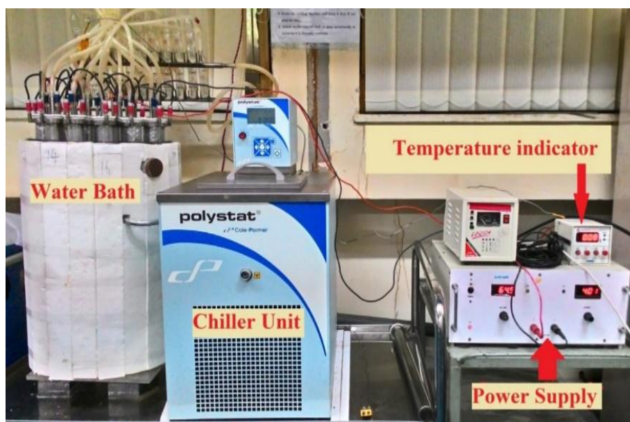
Fig. 4 ELECTROLYSIS SETUP FOR TRITIUM ENRICHMENT
