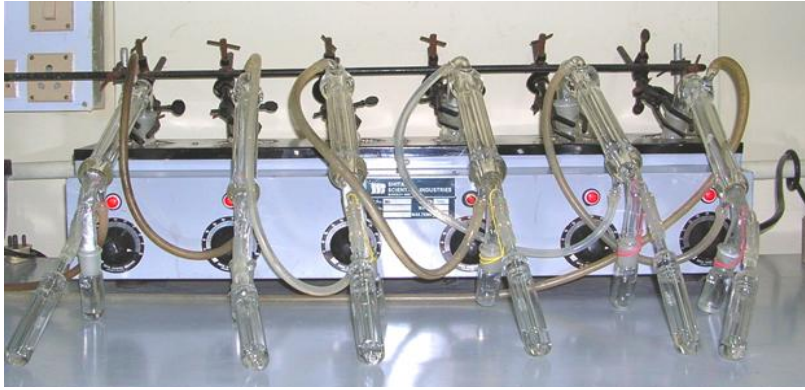
FIG. 5 NEUTRALISATION SETUP FOR SAMPLES POST ELECTROLYSIS
