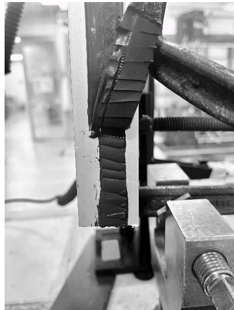
FIG. 9 ADHESION-IN-PEEL TEST SPECIMEN SECURED IN TENSILE MACHINE
