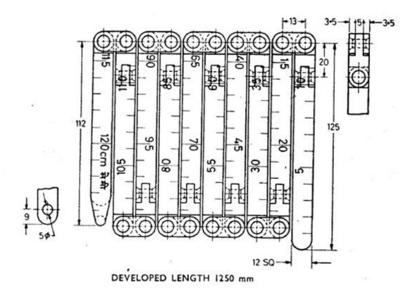
FIG. 1 Dimensions for Flexible Sounding Rods
