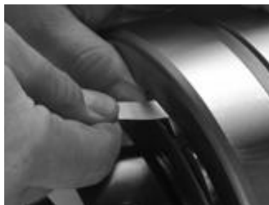
FIG. 15 CHECKING DIAMETRIC SLACKNESS BY FEELER GAUGE
