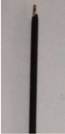
Defect – Top Chip Off
