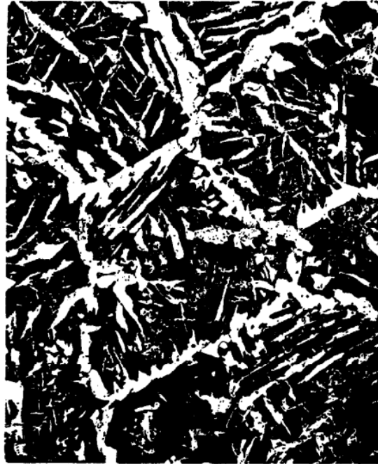
FIG. 13 COARSE GRAIN STRUCTURE DUE TO OVERHEATING
