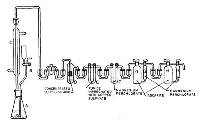
NOTE - Tubes are compactly arranged along the edge of  $150 \times 230$  mm board which is supported 130 mm from the table-top upon a tripod base.
