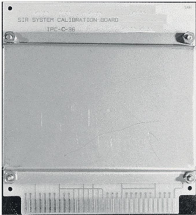
Figure 12 Resistor verification board with protective cover
