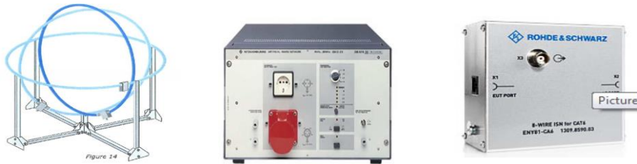
Fig. 17 Typical Magnetic Loop Antenna, Line Impedance, Impedance Stabilization Network & EMI Receiver
