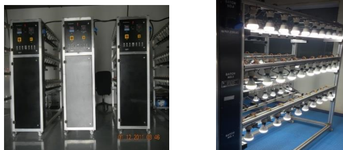
Fig. 22 Typical Life Test Rack for Lamps
