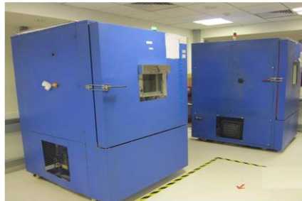
Fig. 21 Typical Humidity Chamber
