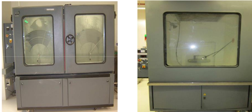
Fig. 14 Typical Dust & Rain Chamber
