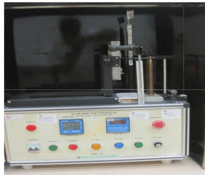
Fig. 19 Glow Wire Test Set Up
