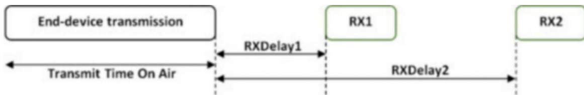
Fig.7 Bidirectional Communication between End-Device and Base Station for LoRaWAN Class A
