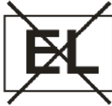
Fig. 5 Lamps Not Suitable for Emergency Operation
