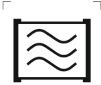
Fig. 1 Lamp Suitable for High Frequency Operation
